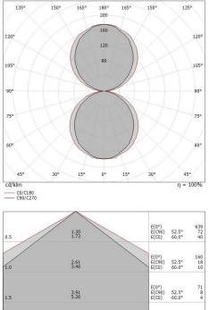
E(0°) E(C90) E(C0) 7.82 10.39 Cone diameter [m 3.0 Distance [m] C0/C180 (Half-peak divergence: 120.0°) C90/C270 (Half-peak divergence: 105.0°)
