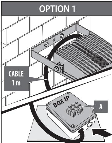
**GB** WARNING: make sure that the connection is made with components that guarantee the IP rating.
